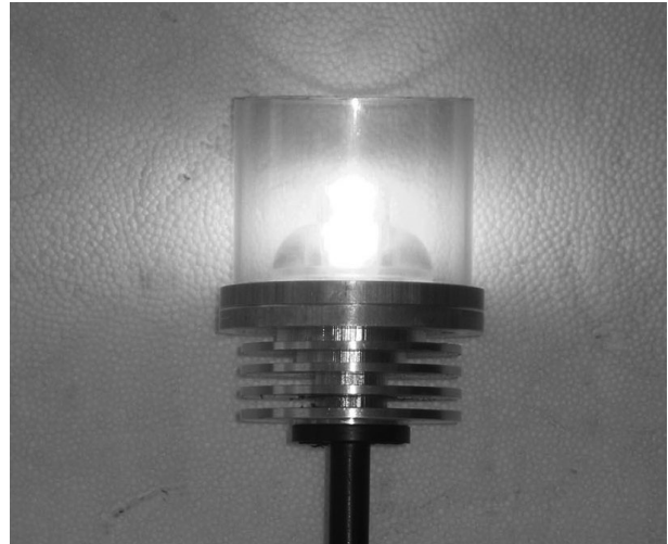
Fig. 5. Appearance of the Y-244 B1 type radiator (for navigation sign lights of water storage basins and lakes)
