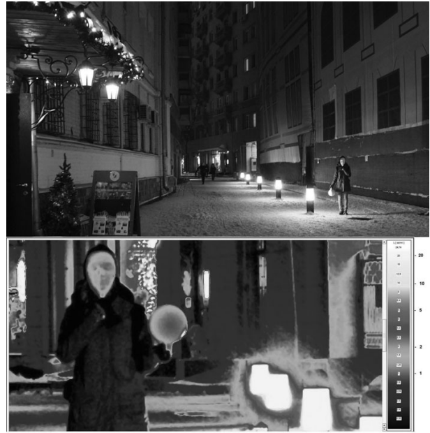
Fig. 4. Ordynskiy cul-de-sac. An uneven light distribution, “footlights effect” with snow, a bad shadow forming effect and an unsettling atmosphere
