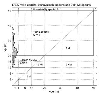
Fig. 4. Vertical Stanford diagram
