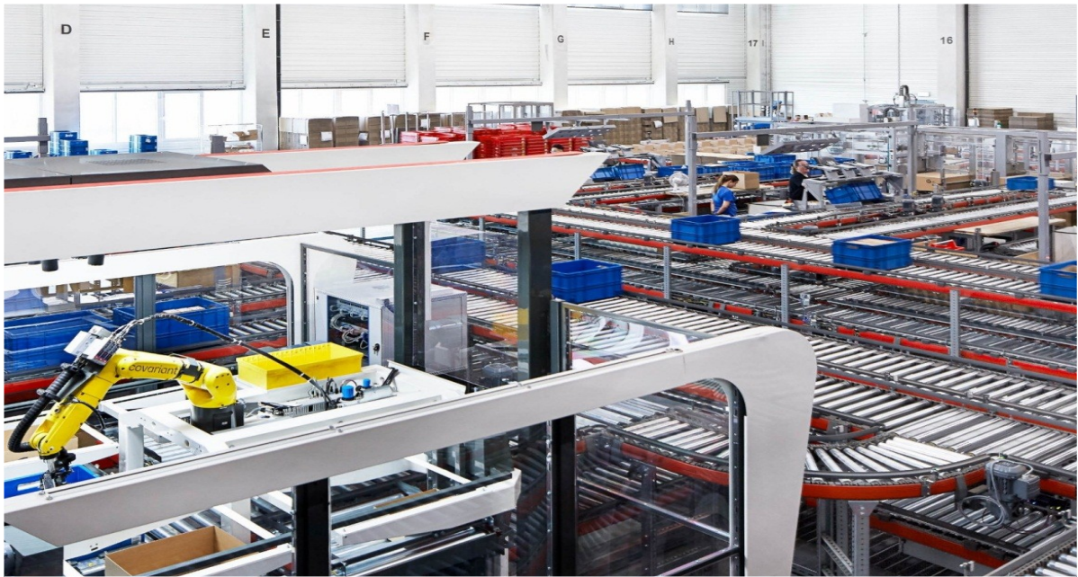
Fig 1.1 Covariant’s robot arms can pick up and sort items of different shapes and sizes
