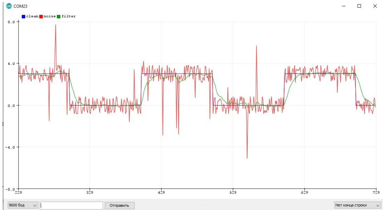
Fig. 4.15. Simple Kalman filter with a step signal
