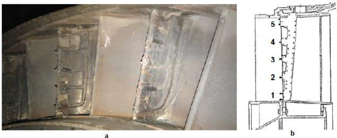
Fig 2.1 - Prepared nozzle apparatus turbofan engine (a); thermocouple layout (b)
