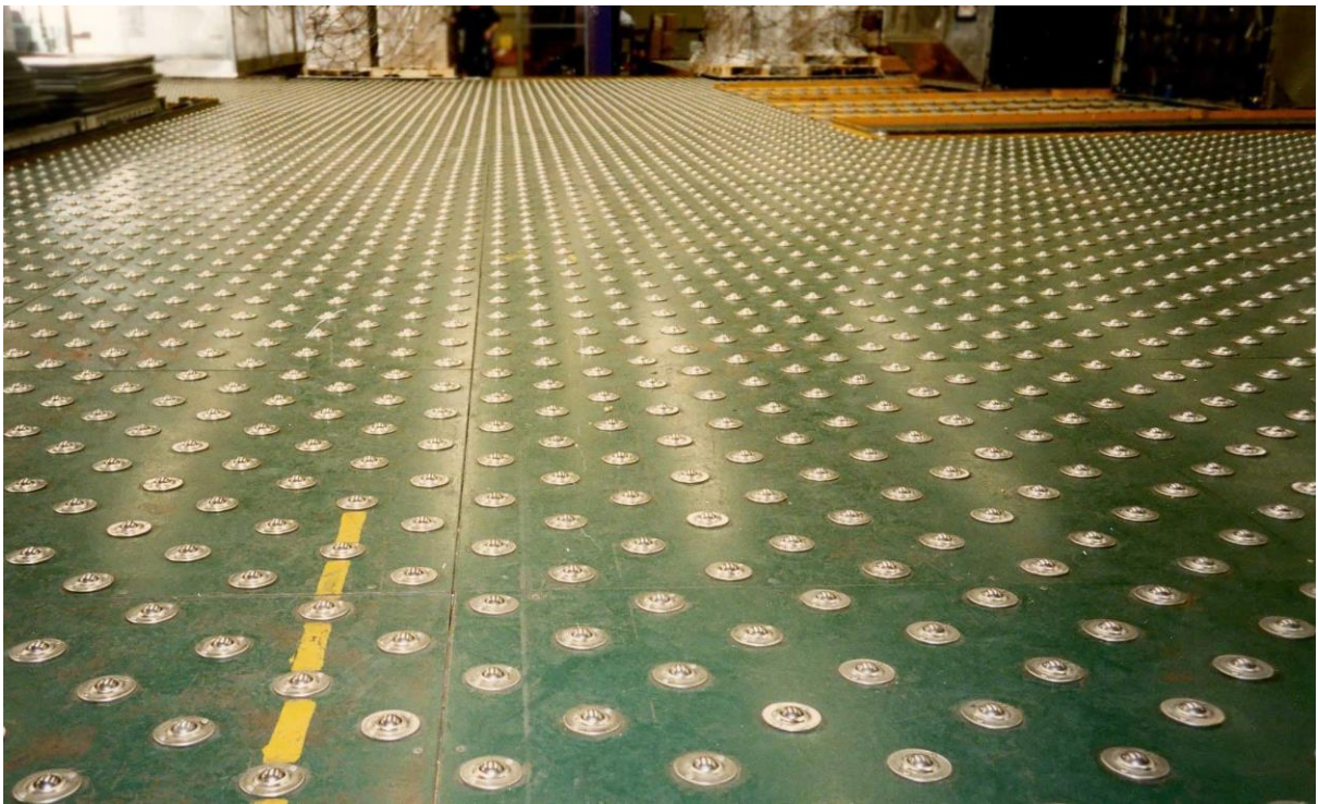
Fig.1.7 - A typical example of ball mat flooring
