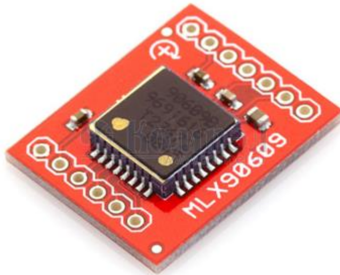
Fig. 3.5.1. The MLX90609 gyroscope is manufactured by Melexis
