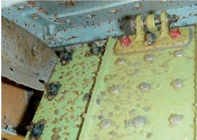
Fig. 15 Residue in gel form on the elevator balance panel of a 737-800 airplane
