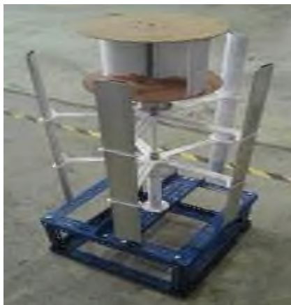
Fig. 5. Hybrid rotor with five blades H-type Darrieus and Savonius on the top
