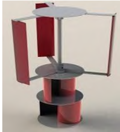
Fig. 6. Hybrid rotor with 3 blade H-type Darrieus and double rotor Savonius below
