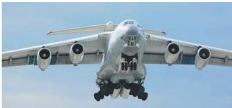
Figure 1.1 – Massive and very important parts of Ил-76 and modern landing gear of transport and passenger aircraft of Ilyushin constructional bureau made of titanium alloy BT22
