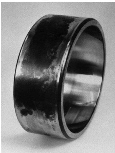
Figure1.15 – Fretting-corrosion of the bearing
