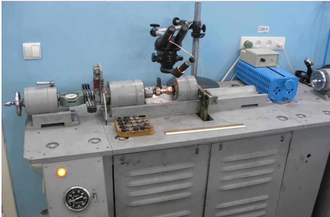
Figure 2.2 – General view of installation for testing the fretting
