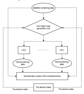
Fig. 1. Structure of the automated system for aerospace monitoring of forest fires
