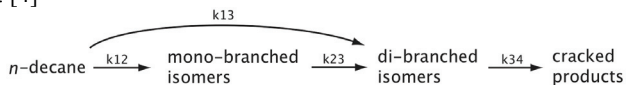
Fig. 1. Proposed reaction scheme of the isomerization of n-decane with reaction path of direct di-branching k13
