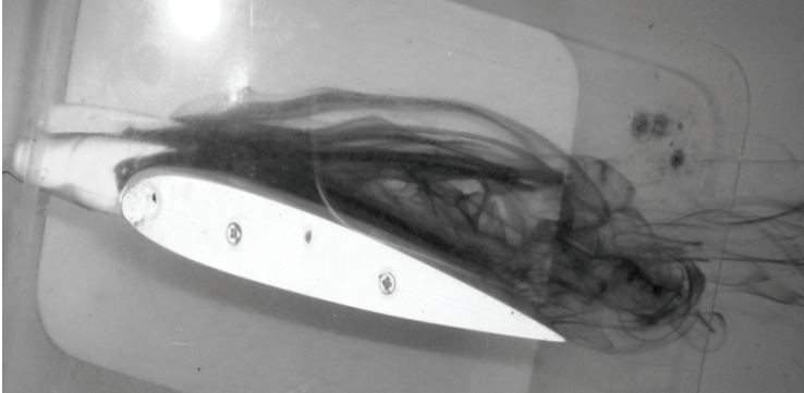
Fig.2 A part of unsteady flow over the wing with vortex generator on the leading edge, \alpha=15^\circ
