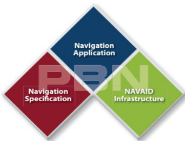
Figure 4. Components of PBN Concept
