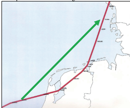
Figure 1. ATS Routes Straightening within Free Route Airspace
