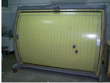
Fig. 5. An experimental stand for measurement of sound-proofing of aviation panel
