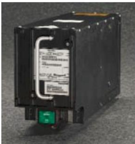
Fig. 4.3. Appearance and main characteristics of HG2030BE ADIRU [8]
