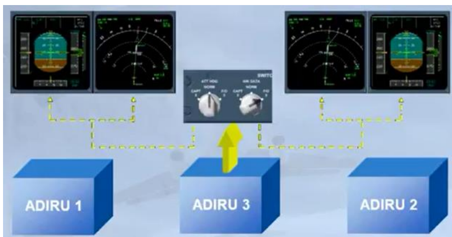
Fig. 4.6. ADIRU № 3 is a standby unit [9]
