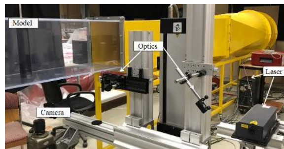
Fig. 1. Particle Image Velocimetry arrangement for the experiments
