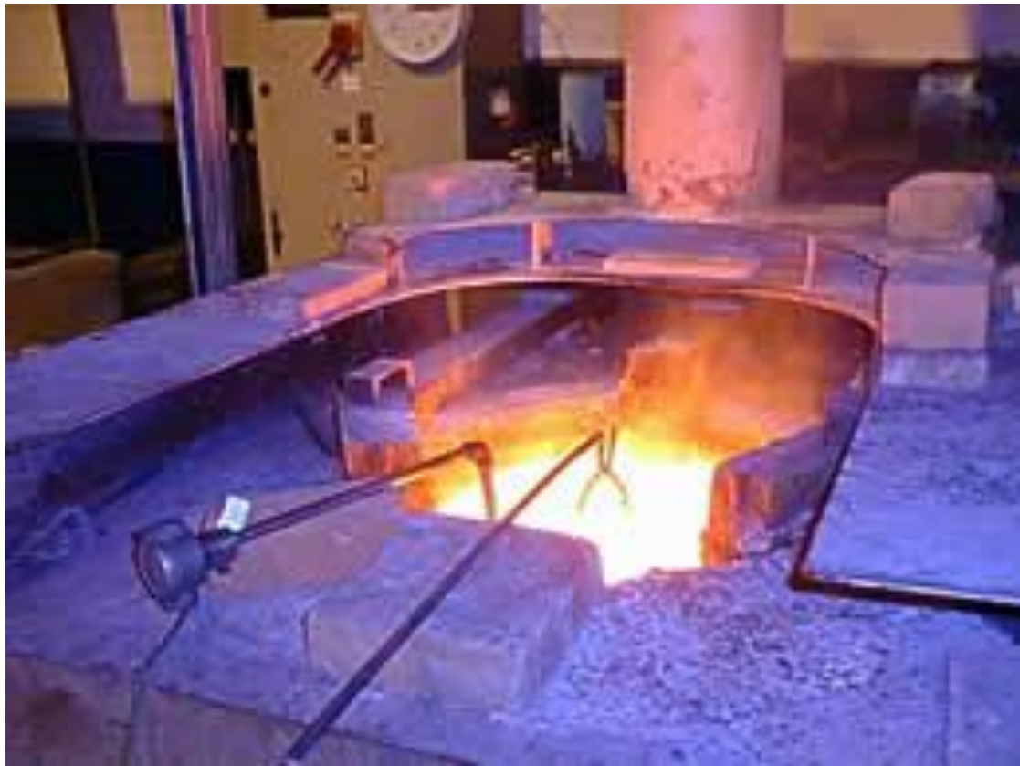
Salt bath nitriding process
