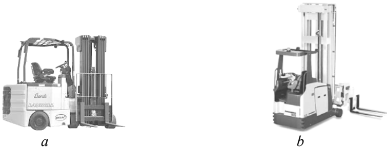
Fig. 7. Basic types of narrow aisle trucks: a – swing mast truck; b – turret truck
