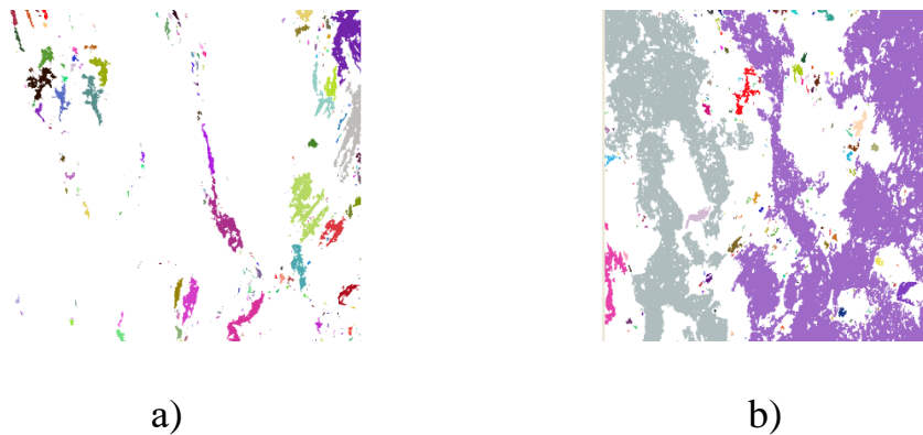
Figure 3.14 - Clusters of deformation relief: a) N = 47300 cycles - the first stage;
