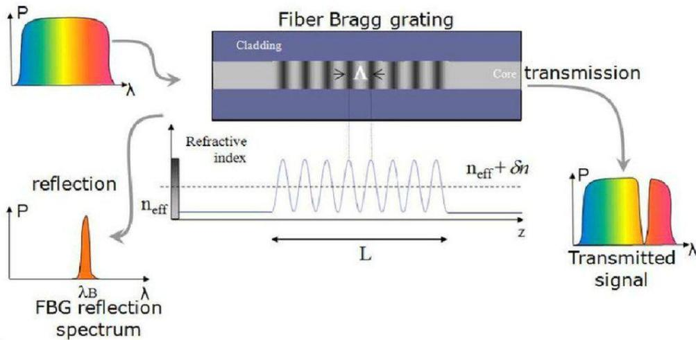
Figure 3.31 - Fiber Bragg grating principle of operation
