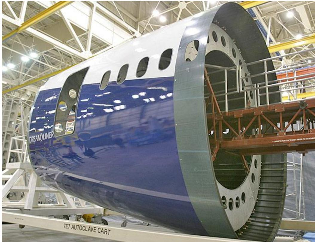
Figure 2.29 - Aircraft fuselage made of carbon fibre epoxy composite
