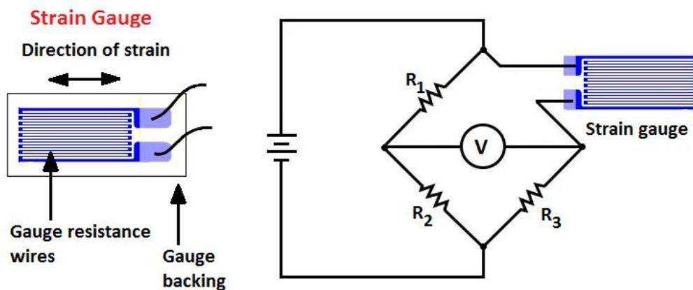
a) Strain gauge b) strain gauge functional diagram
