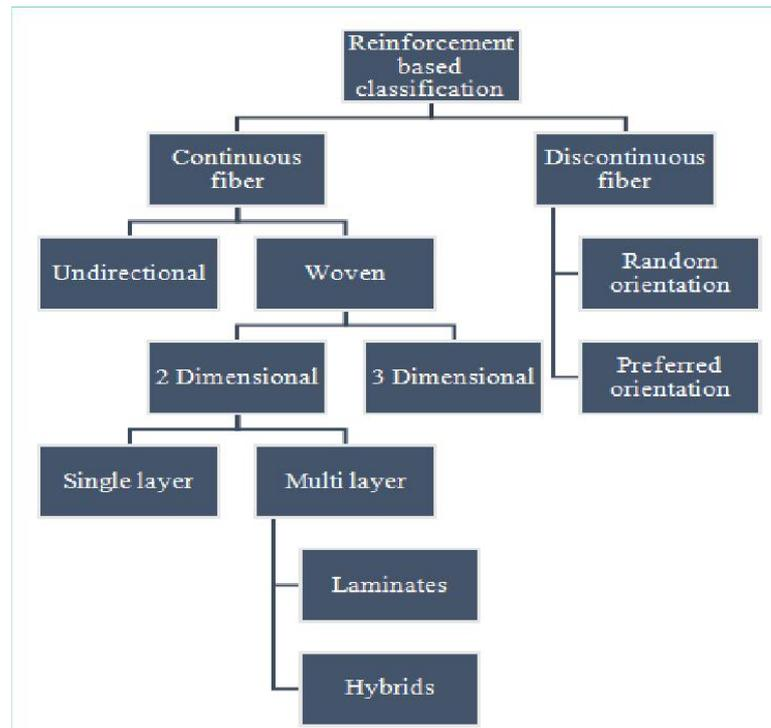
Figure 1.5 - Classification of fiber reinforcement
