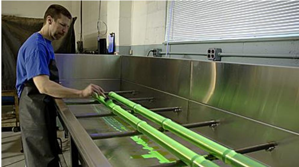
Figure 2.21 - Fluorescent liquid penetrant inspection
