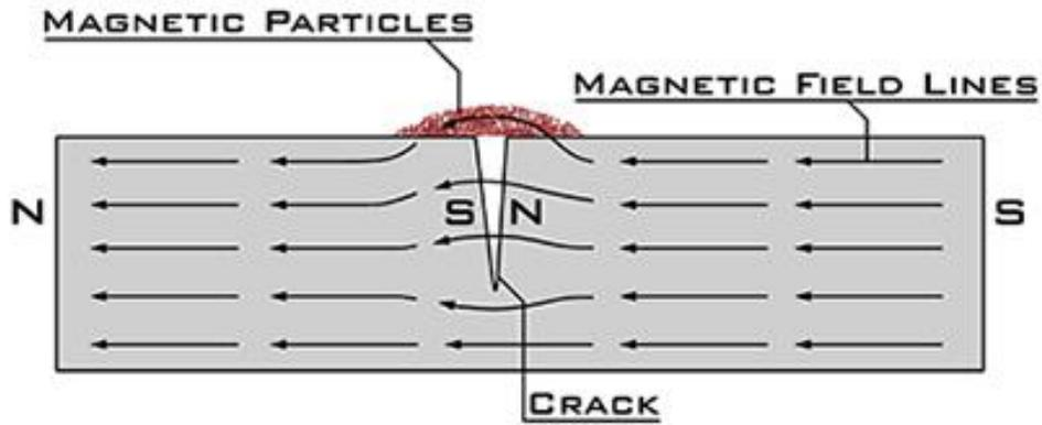
Figure 2.18 - Colour contrast magnetic particle inspection technique
