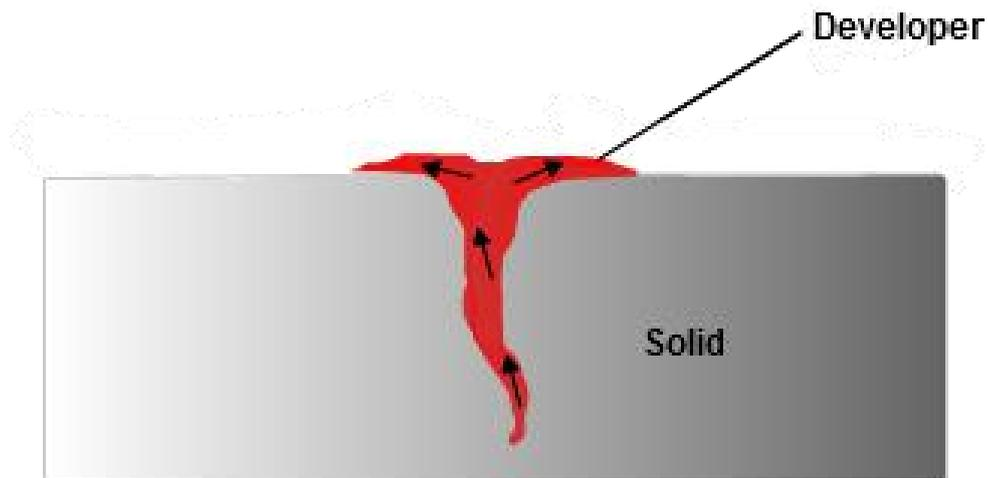
Figure 2.20 - Representation liquid penetrant inspection technique
