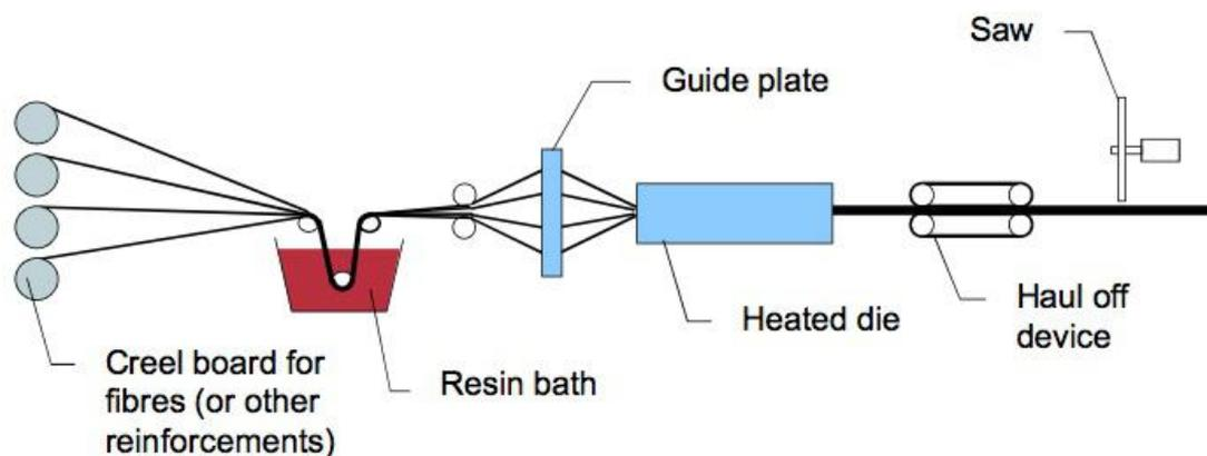
Figure 1.10 - Pultrusion technique for fabrication of fibrous composites
