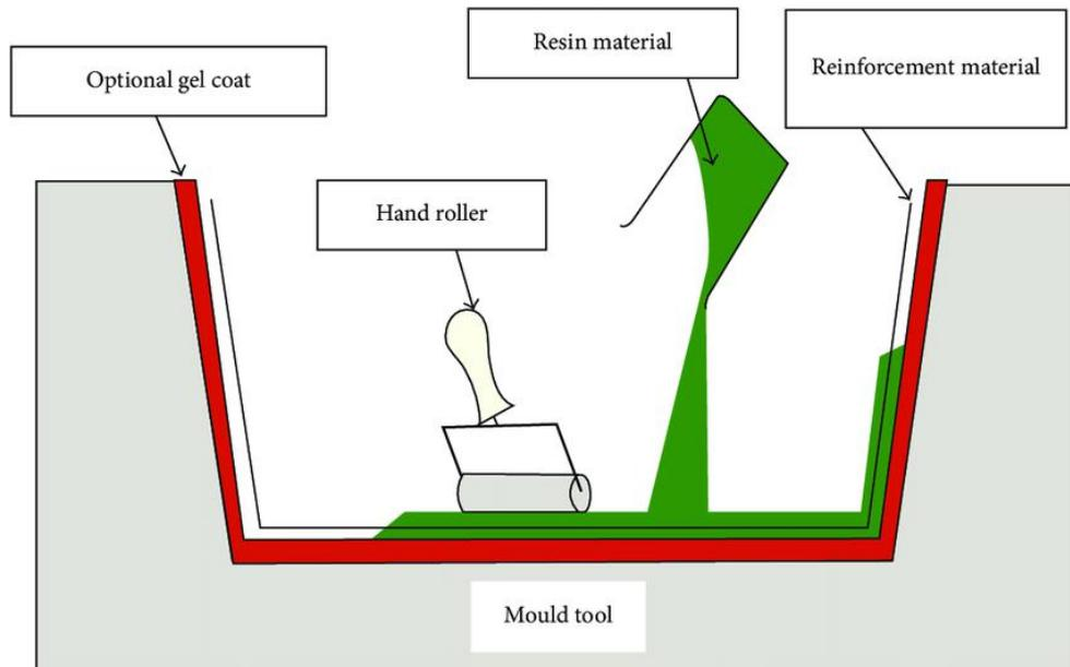
Figure 1.12 - Hand layup fabrication technique
