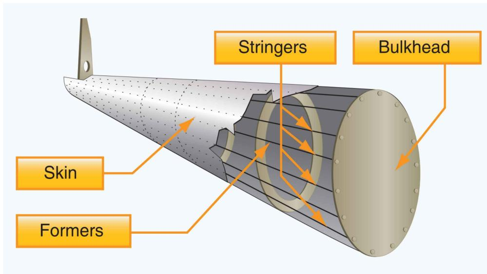
Figure 1.2 - Semi monocoque fuselage configuration
