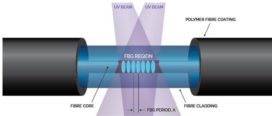
Figure 3.30 - Fiber optic sensor representation
