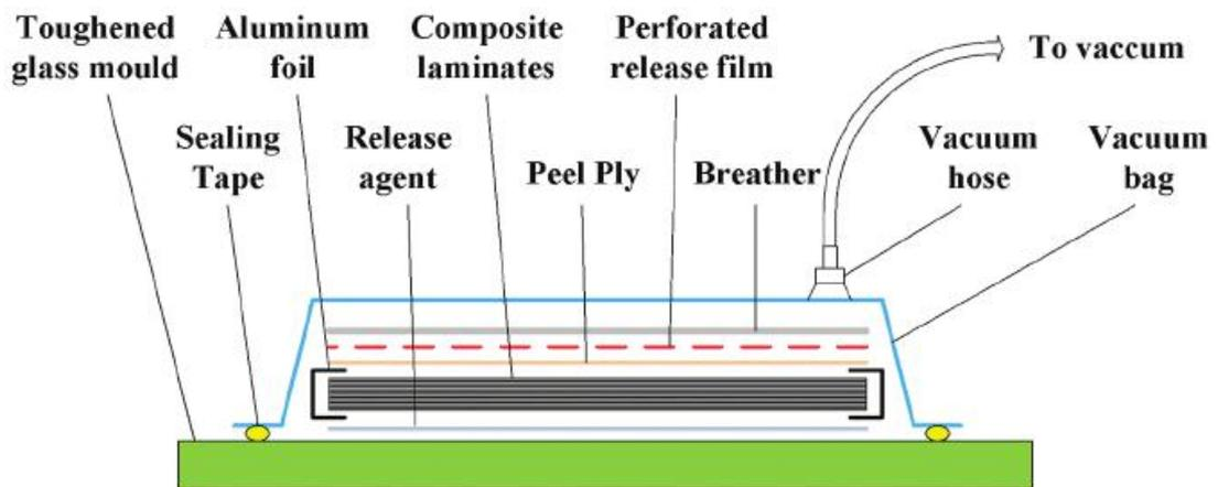
Figure 1.11 - Vacuum bagging fabrication method
