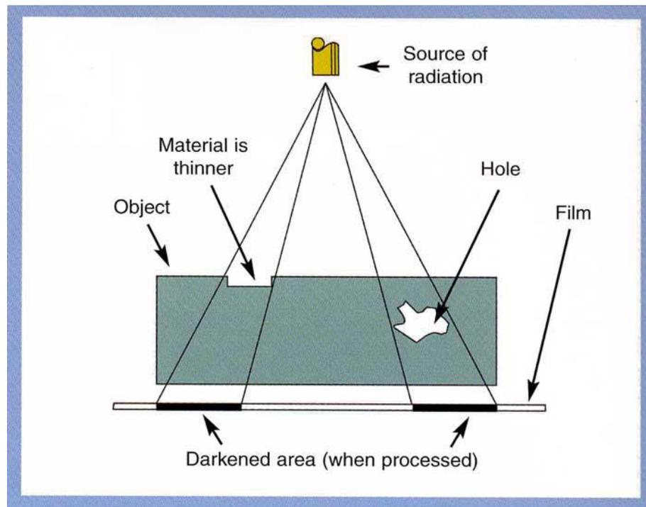
Figure 2.27 - Radiographic inspection technique representation
