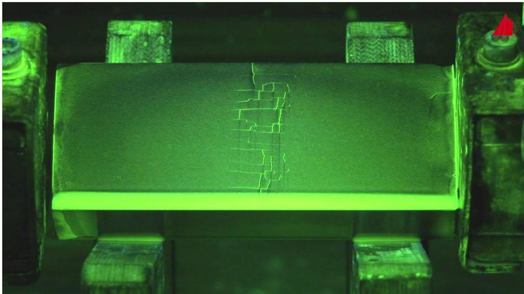
Figure 2.19 - Magnetic particle fluorescent inspection
