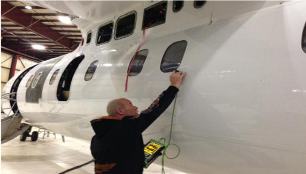
Figure 2.17 - Fuselage inspection using ultrasonic diagnostic
