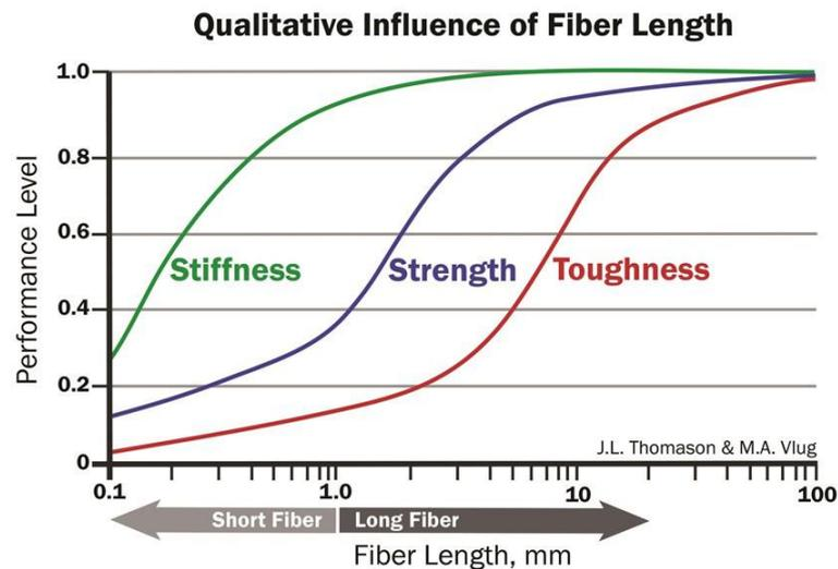
Figure 1.6 - Influence of fiber length on mechanical properties
