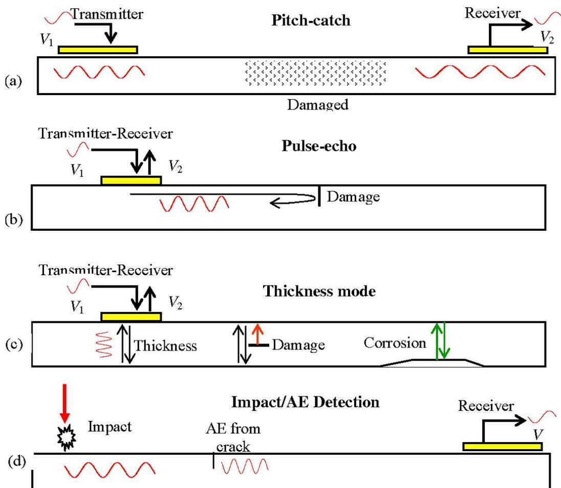
Figure 3.33 - Functional process of the piezoelectric wafer active sensors
