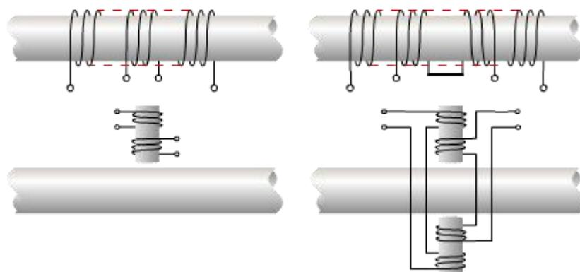
Figure 2.23 - Representation of the absolute mode of operation
