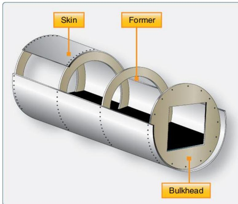
Figure 1.1 - Monocoque fuselage configuration
