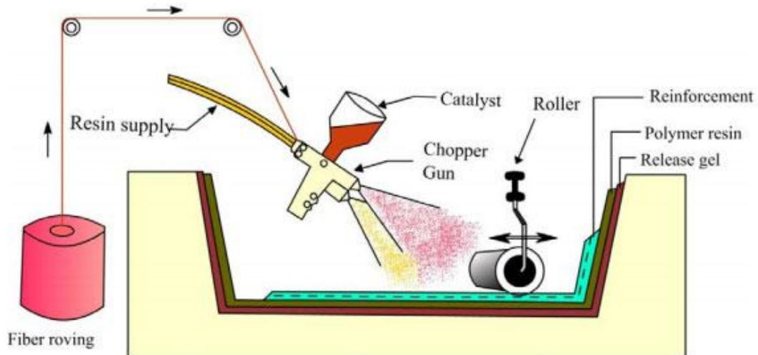
Figure 1.9 - Spray layup fabrication method
