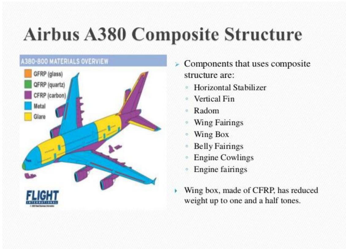
Figure 2.28 - Increasing percentage of composite materials in aircraft structure
