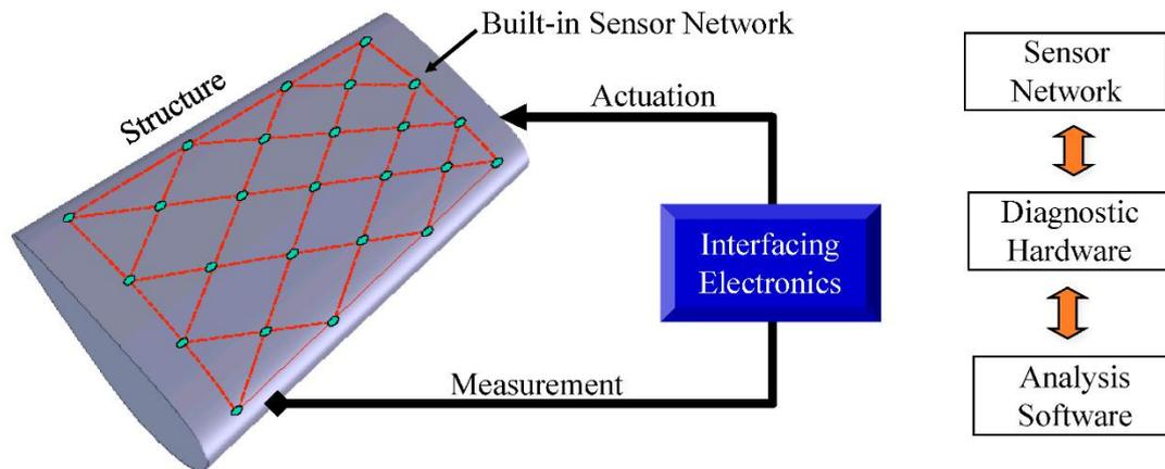
Figure 3.34 - Example of damage detection using the piezoelectric wafer active sensors
