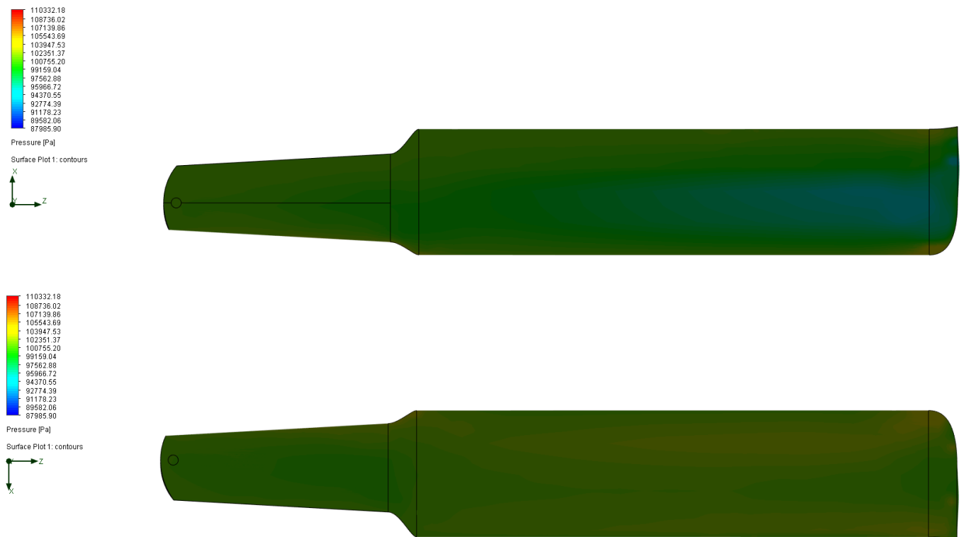
Figure 3.15. Pressure distribution in hovering mode
