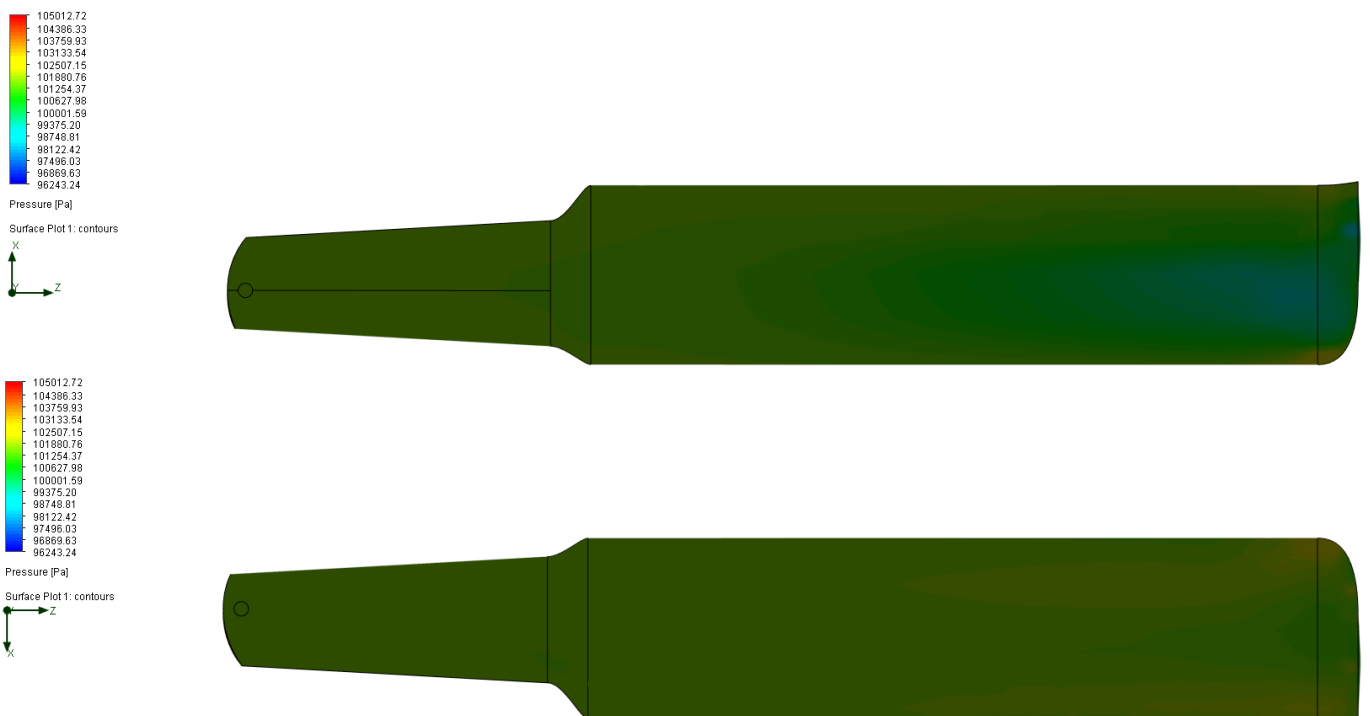
Figure 3.19. Pressure distribution on retreating mode
