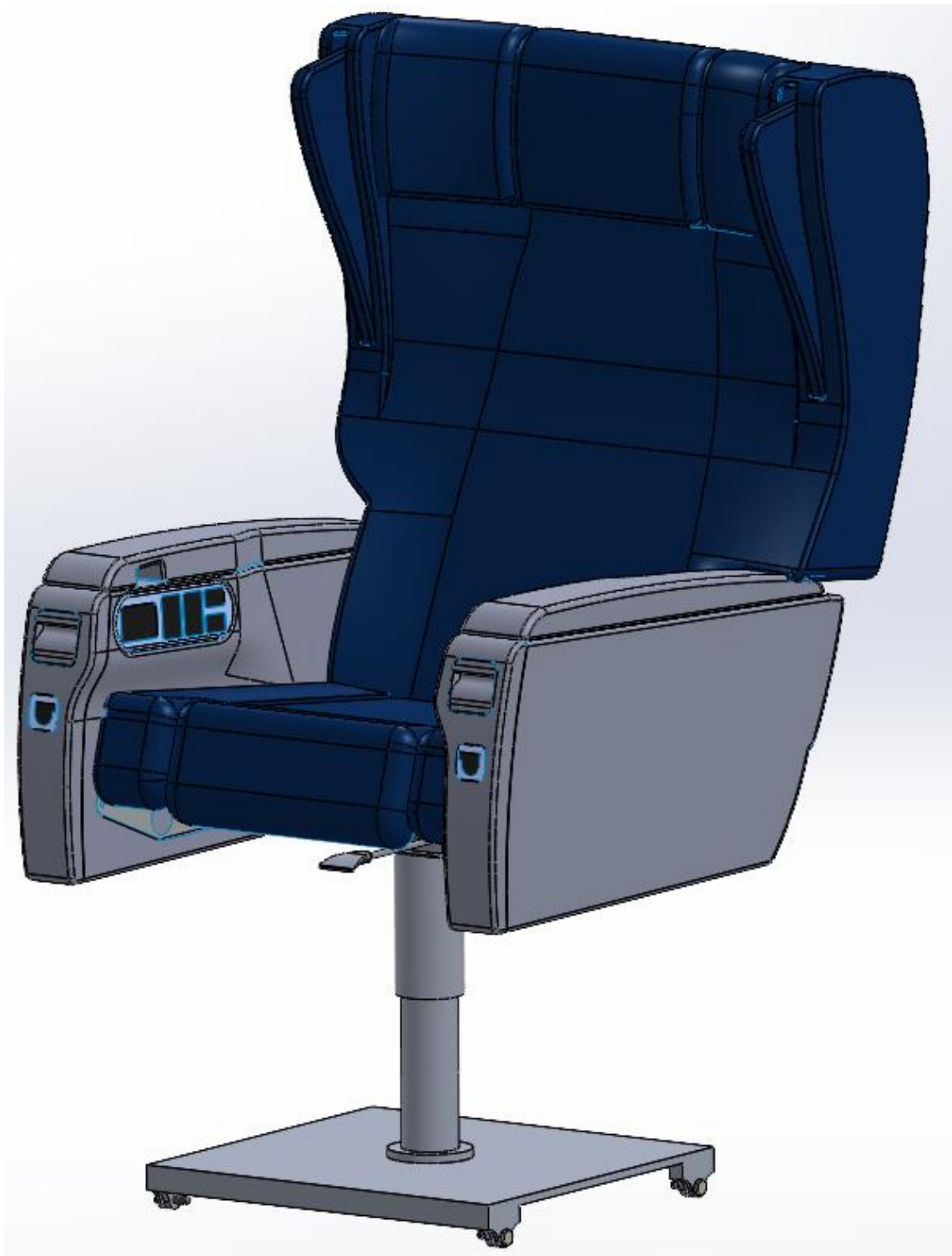
Fig. 3.29. General view of the passenger seat with built-in gas lift.
