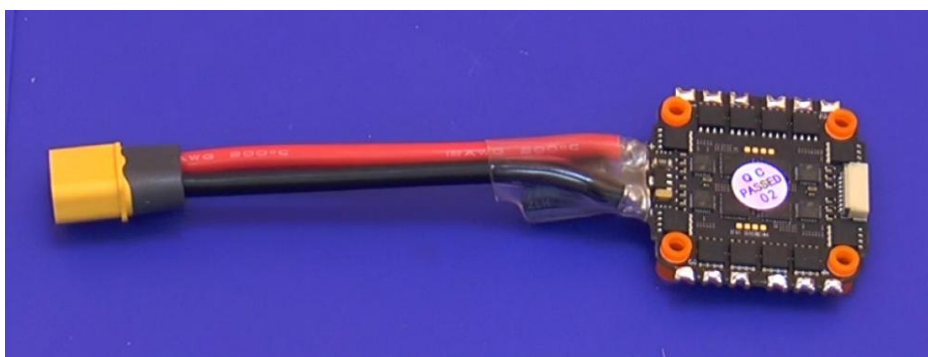
Fig. 4.5 Solder the power wires to the ESC
