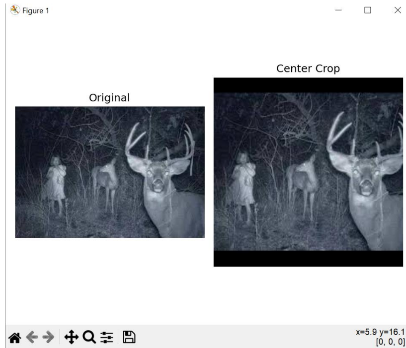
Fig. 2.18. Visualisation of an example using the the Centre Crop method
