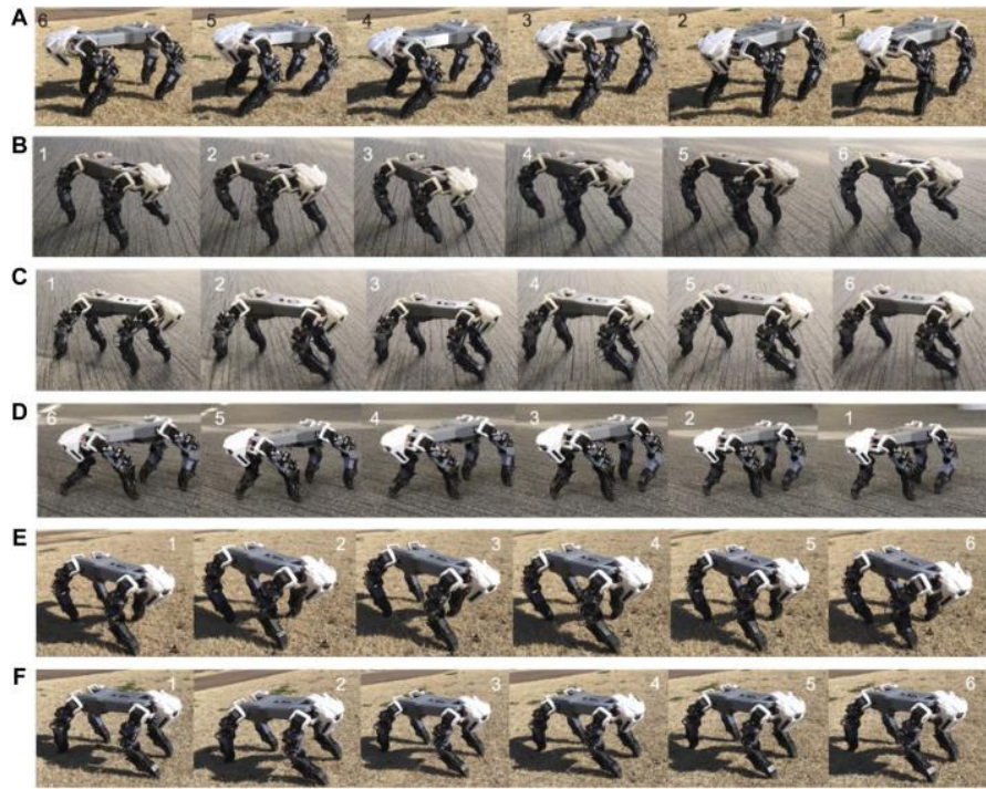
Fig. 2.2 The robot's dynamic gait pattern (A) on natural terrain (B) on flat terrain. (C) Dynamic gait pattern on flat terrain with injured forelimb. (D) On flat terrain with injured hindlimb. (E) On natural terrain with injured forelimb. (F) On natural terrain with injured hindlimb.
