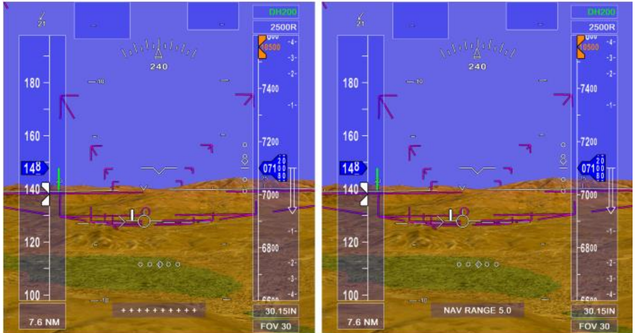
Fig. 3. The SRS box awaiting spoken command (left) and displaying the recognized command(right).
