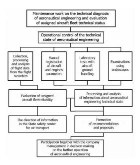
Fig. 2. Functional diagram of the aircraft maintenance system
