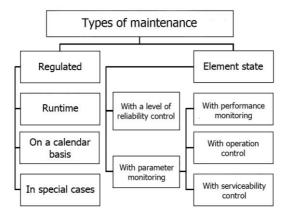
Fig. 1. Classification of maintenance types
