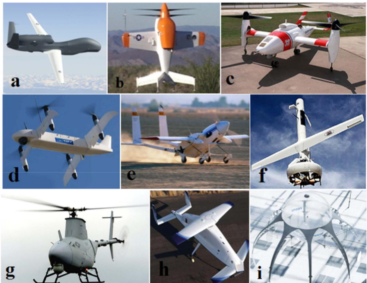
Fig. 2.6. Different types of UAVs, (a) HTOL [28], (b) VTOL [29], (c) tilt-rotor UAV [30], (d) tilt-wing UAV [31], (e) tilt-body UAV [32], (f) ducted fan UAV [33], (g) helicopter [34], (h) heli-wing [35], and (i) unconventional UAV [36].
