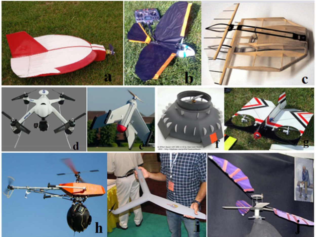
Fig. 2.8. Different types of MAVs, (a) fixed wing, (b) flapping wing, (c) fixed/flapping-wing, (d) rotary wing , (e) VTOL, (f) ducted fan, (g) tilt-rotor, (h) helicopter, (i) unconventional, (j) ornicopter.
