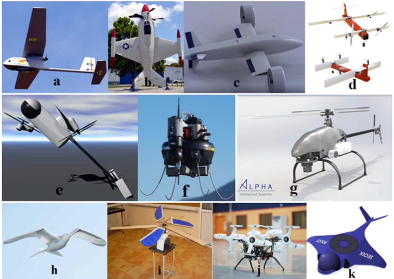
Fig. 2.7. Different types of \mu UAVs, (a) HTOL, (b) VTOL, (c) tilt-rotor, (d) tilt-wing, (e) tilt-body, (f) ducted fan \mu UAV [58], (g) helicopter, (h) ornithopter, (i) ornicopter, (j) cyclocopter, and (k) unconventional \mu UAV.
