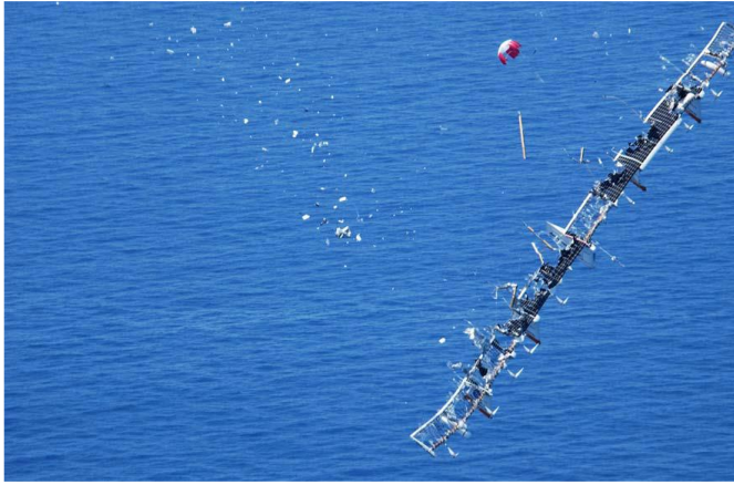
Fig. 9. Helios HP03 unmanned aerial vehicle crash (July 26, 2003).
