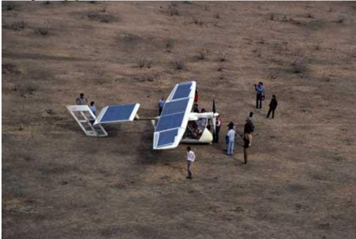
Fig. 4. Manned Aircraft "Solar Challenge" Powered by Solar Cells.
