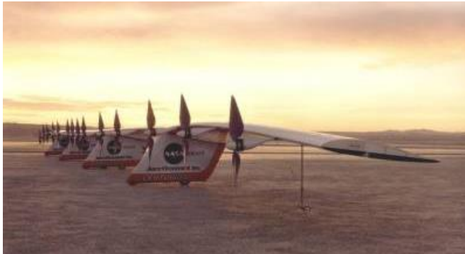
Fig. 6. Unmanned high altitude aircraft platform (aircraft -prototype Centurion, USA).
