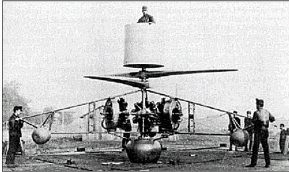
Fig. 1. Helicopter PKZ-2 on electric propulsion (1917).
