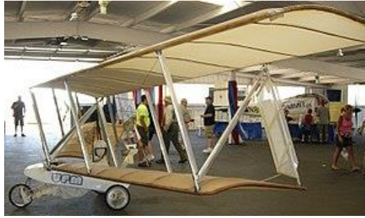
Fig. 2. The Mauro Solar Riser piloted aircraft is powered by a SC – battery.
