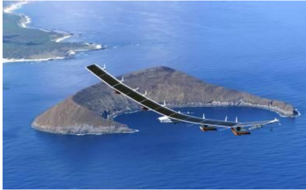
Fig. 8. Helios unmanned aerial vehicle Helios HP03 after takeoff (Kauai Island, Hawaii, USA).
