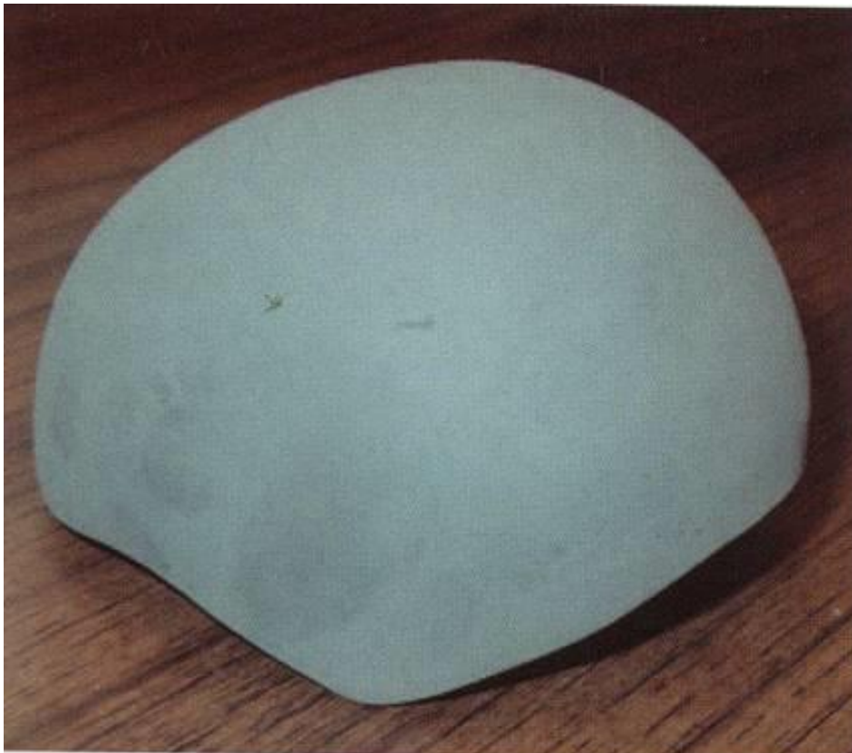
Figure 1.5 – A new boron carbide shaping process creates complex curved shapes for use in helmets and other personal protective equipment.
