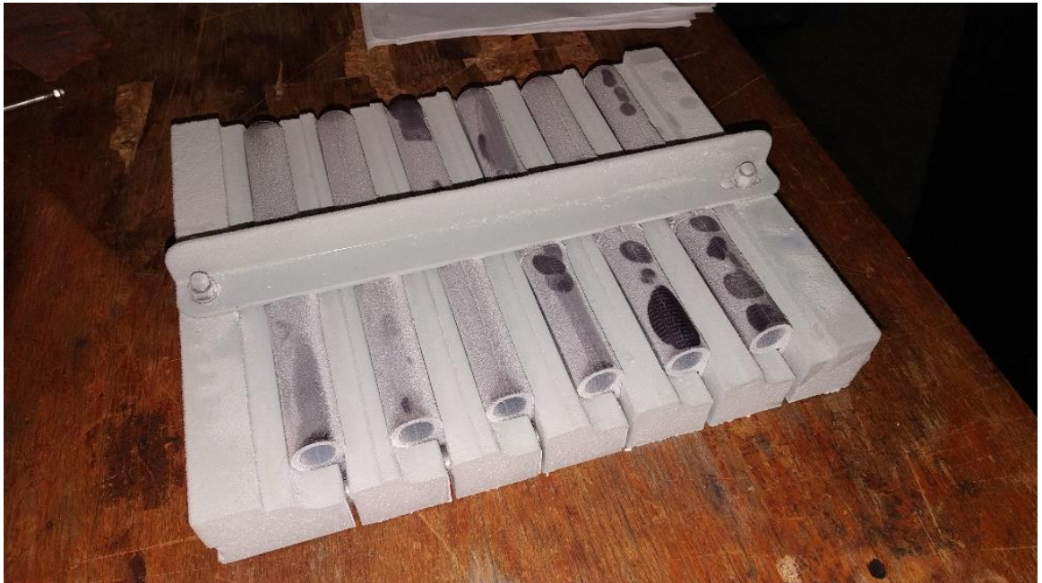
Figure 2.3 - Sealing profiles at thermal testing
