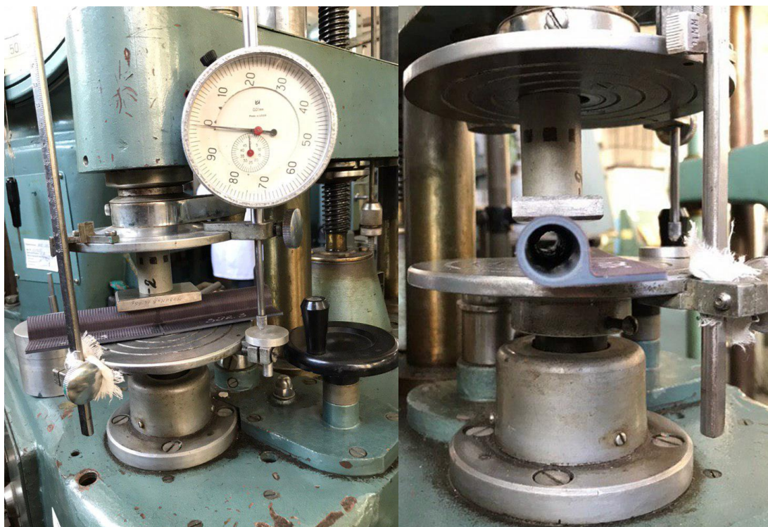
Figure 2.1 - Hydraulic press and sealing profile at testing.
