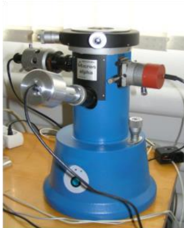
Image 3.1 General view of the developed profilometer created based on the microinterferometer
