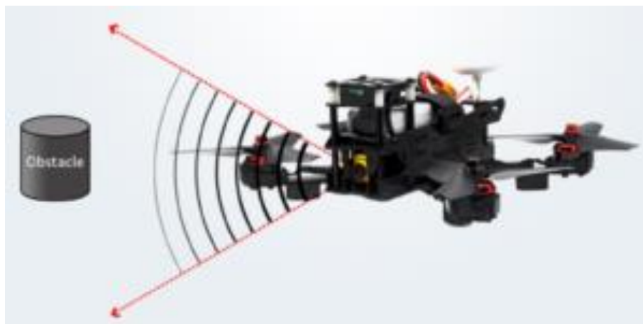
Figure 2.11 – Ultrasonic sensor measuring distance from object during drone’s flight
