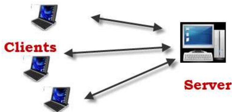
Fig.1.6 Client-server architecture representation
