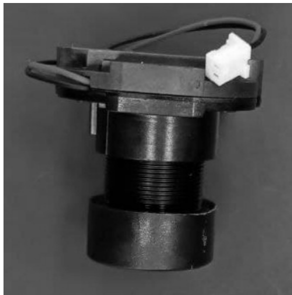
Fig. 2.14 Turn screws into the "TWX5-21-21-41(2024P) M12xP0.5 IR-Cut"
