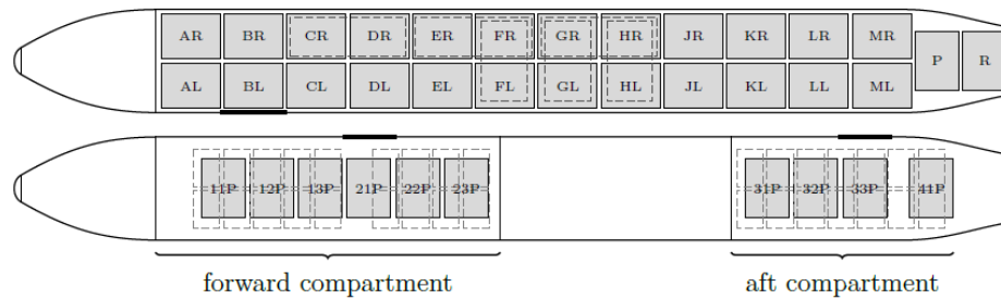
Figure 1.6 - Layout of the loading positions of an MD11F freighter aircraft
