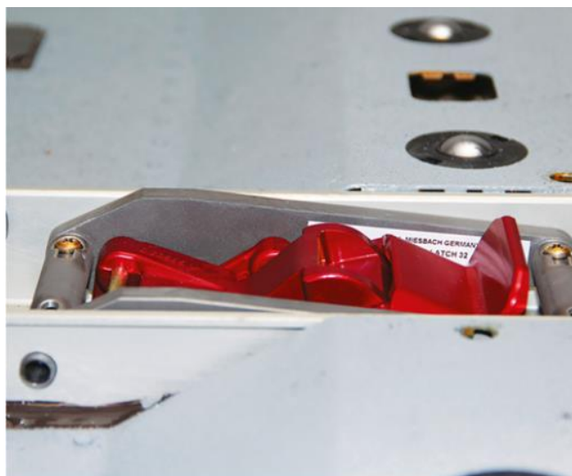
Figure 1.4 - XZ latch in lower position
