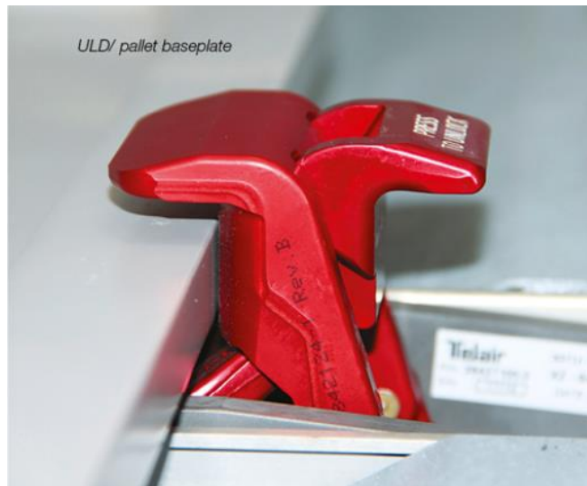
Figure 1.5 - XZ latch in locked position
