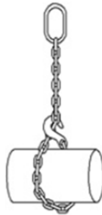
Figure 1.9 - Attachment of tube only with hook
