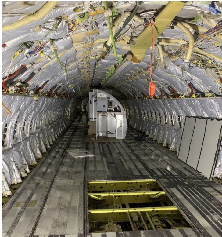
Fig. 1.10 - Inspections areas from STA360 up to pressure bulkhead on practice
