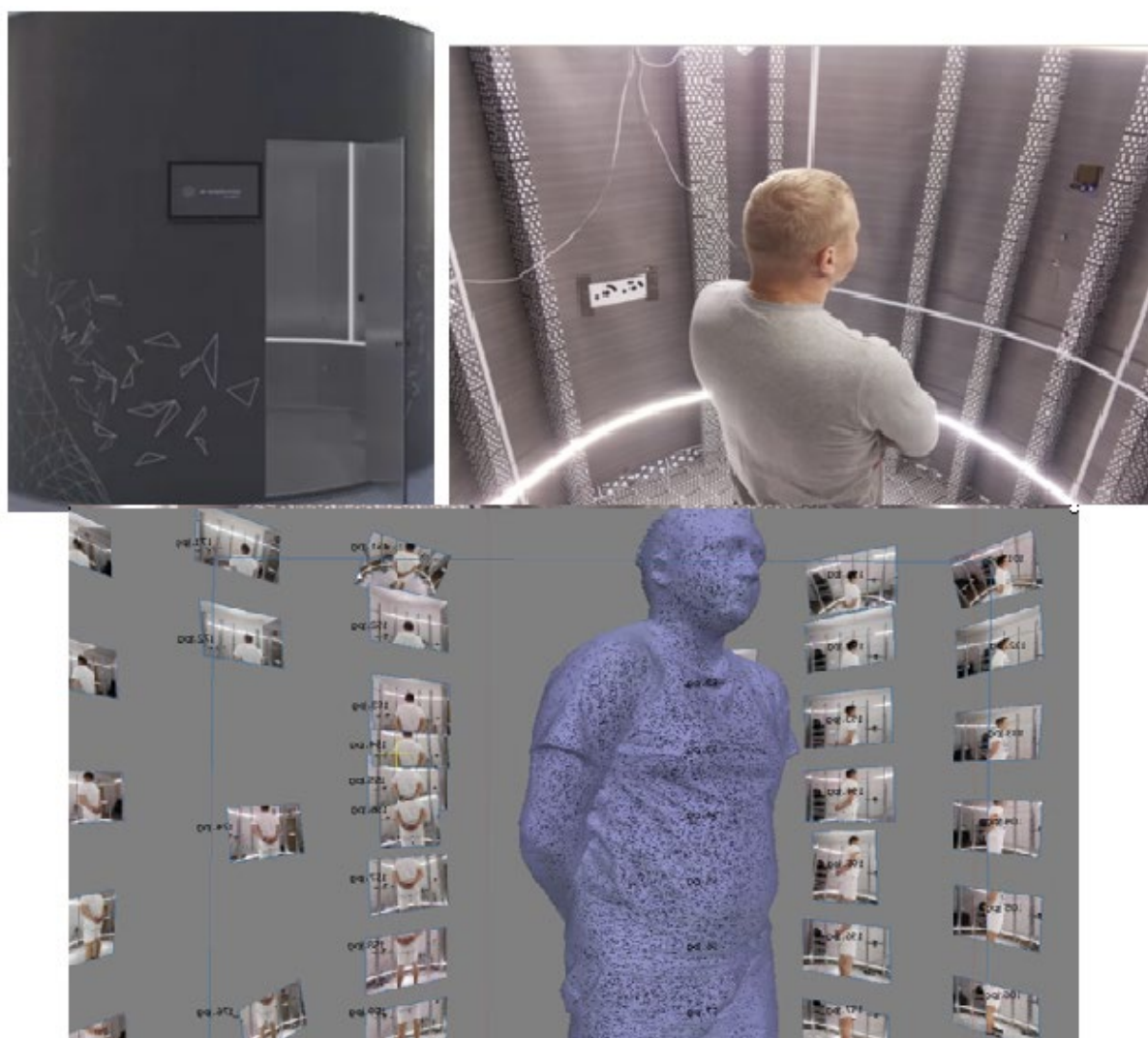
Fig. 6. Panoramic scanners made by 3D GENERATION LLC
