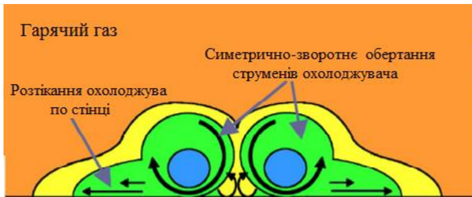
Figure 3.1 - Scheme of the idealized vortex structure of the cooler jet at the flow from the hole of complex shape
