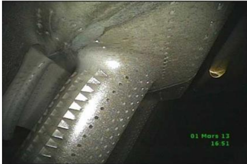
Figure 3.5 - Fan-shaped perforation holes on the nozzle apparatus of the TVT.
