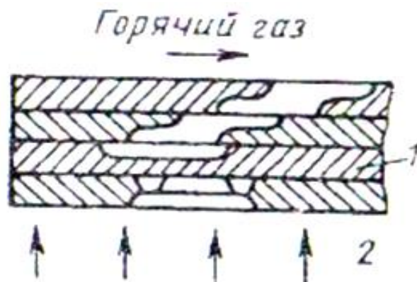
Figure 1.13 - Scheme of multilayer perforated material:
