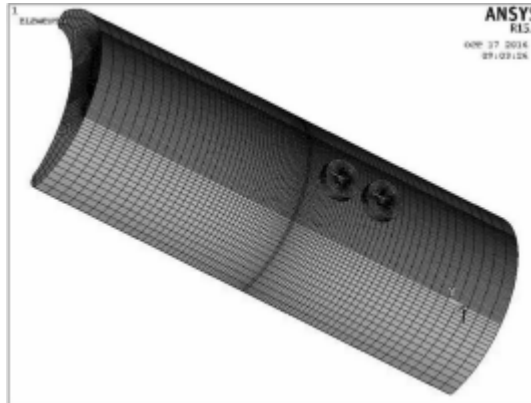
Figure 3.2 Meshing of finite element model of blade body and coil
