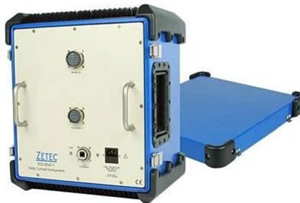
Figure 2.19 Modular Eddy Current Testing Unit
