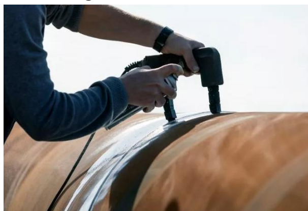
Figure1.5 Magnetic Particle Testing
