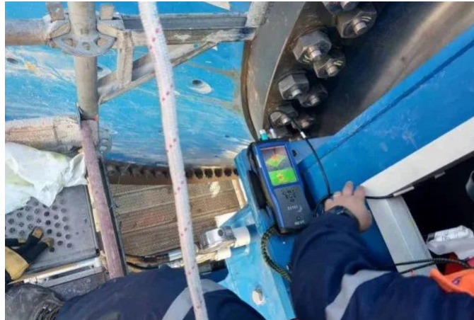
Figure1.7 Eddy current testing
