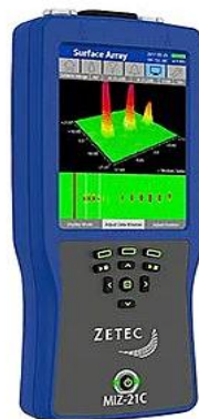
Figure 2.17 Handheld eddy current testing instruments
