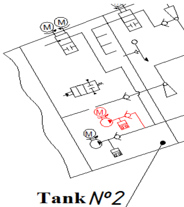
Figure 2.7 – Suggested improvements in tank №2.
