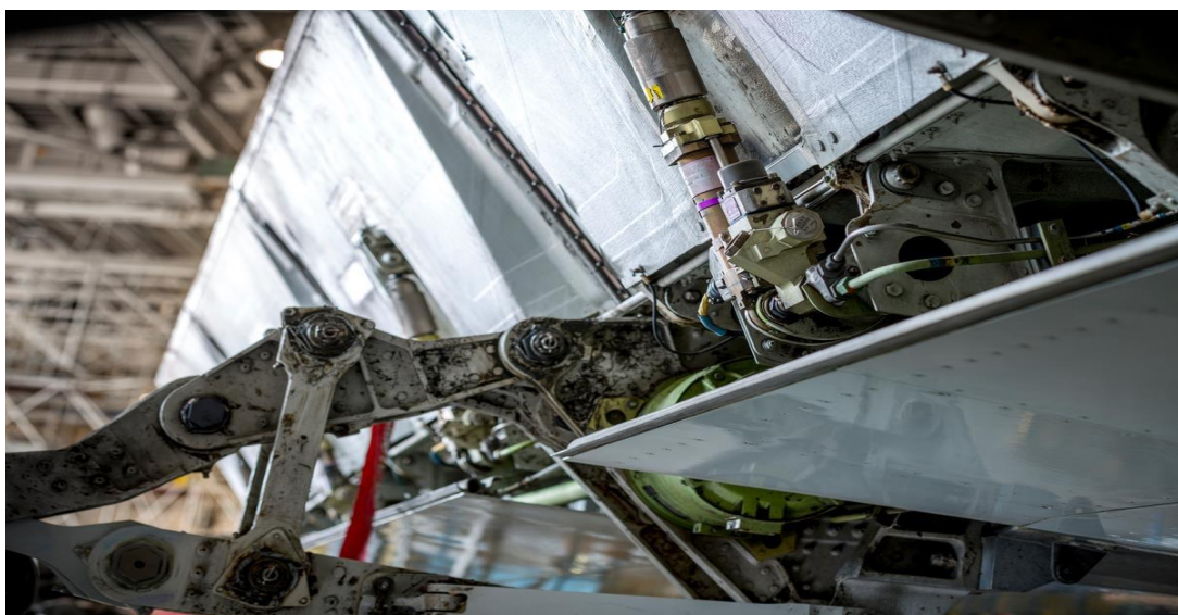
Figure 1.19 - Boeing 737-800 spoilers lubricated with grease AeroShell 33
