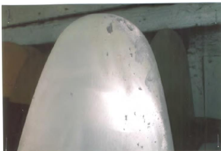
Figure 1.2 - A propeller blade of an AI-24 aircraft engine with a damaged surface
