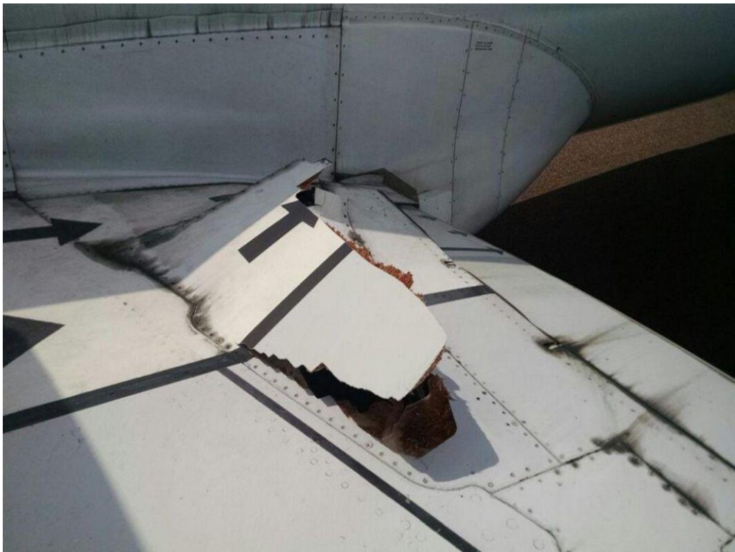
Figure 1.10 – Left hand wing damaged by the shock-strut
