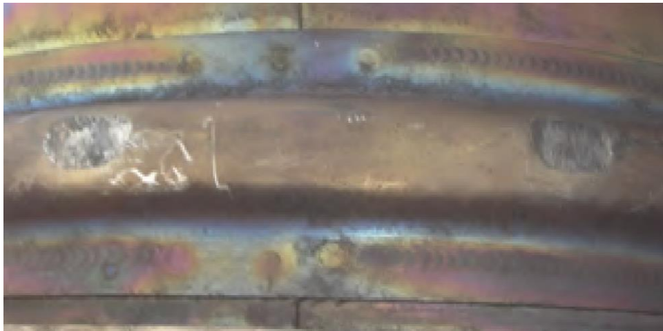
Figure 1.6 - Flame tube showing signs of wear
