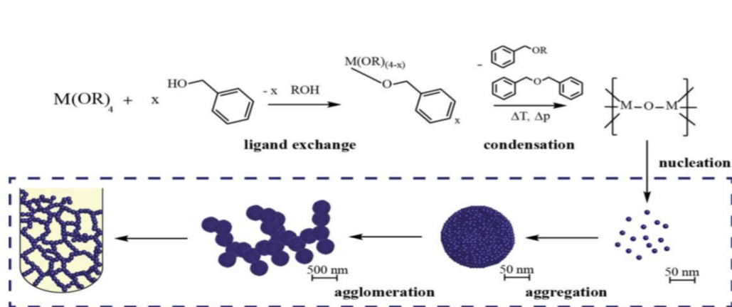
Figure 3.8 - Mechanisms of particle formation in non-aqueous synthesis with an emphasis on the processes of aggregation and agglomeration
