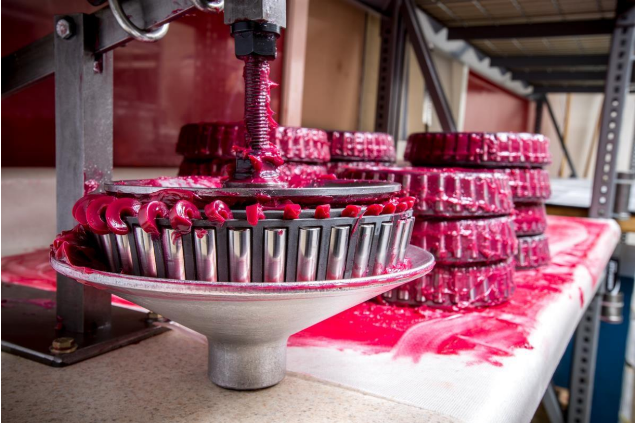
Figure 1.16 - Roller bearings lubricated with plastic grease
