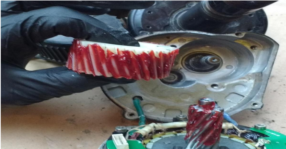
Figure 1.21 - Mobilgrease 28 in a speed reducer
