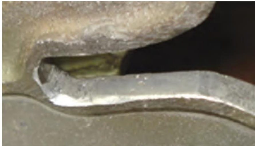
Figure 1.7 - The working surface of the body of the lock of the landing gear of the An-24 aircraft
