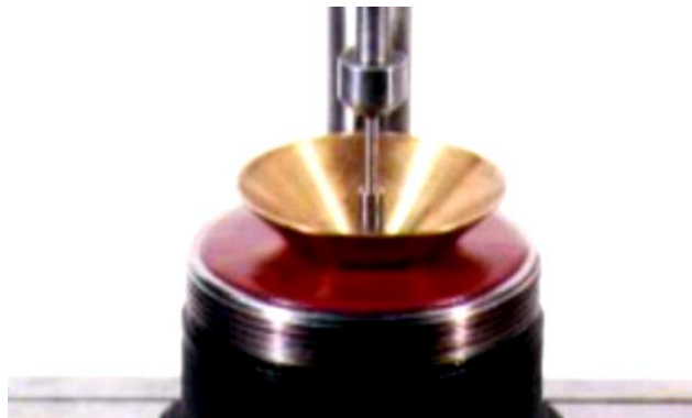
Figure 1.8 - Penetrometer cone released in grease
