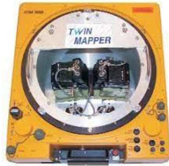
Fig.1.6 TwinMapper installed on a GSM-3000 gyro platform
