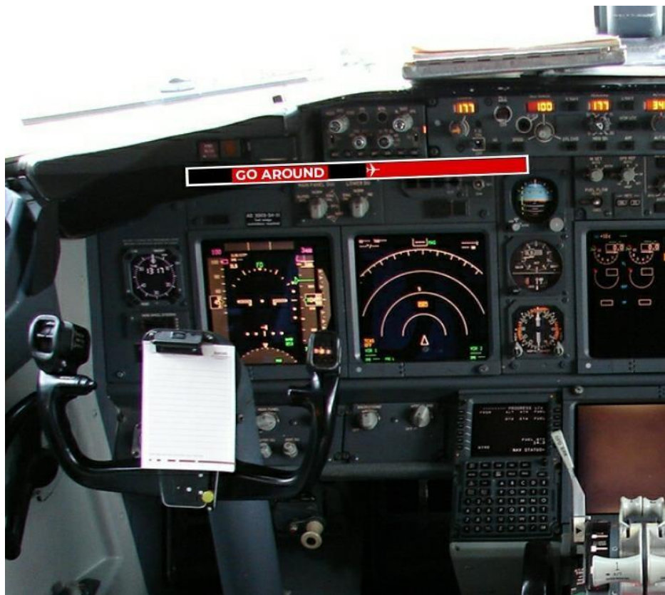
Figure 7: Unsafe landing warning
