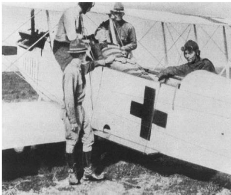
Fig. 3.1. The Curtiss JN-4 Jenny was converted to an air ambulance.
