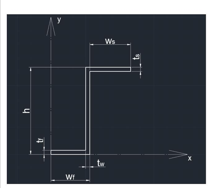
Fig. 3.1. Geometrical characteristic of cross-section of the stringer.w<sub>s</sub>=30 mm; w<sub>f</sub>=28.5 mm; h=65.5 mm; t<sub>s</sub>=3mm; t<sub>f</sub>=3 mm; t<sub>w</sub>=3mm.
