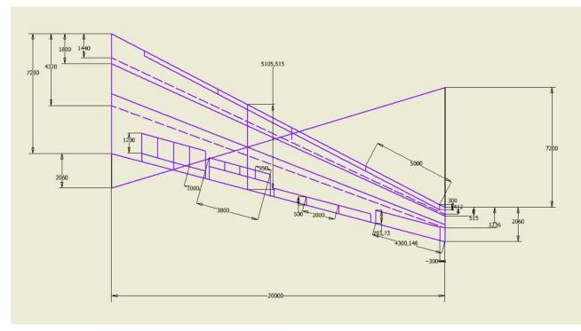
Figure 2.1 Geometrical method of determination mean aerodynamic chord
