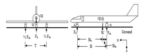
Figure 2.2. Landing gear parameters
