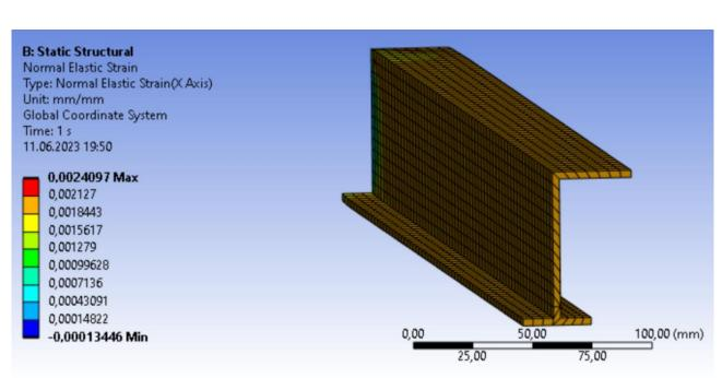
Fig. 3.4. Deformation state of the modified stringer
