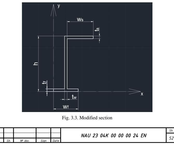
Verification calculation for the modified stringer is being conducted. The calculation should be carried out only for the cab local buckling stress.
