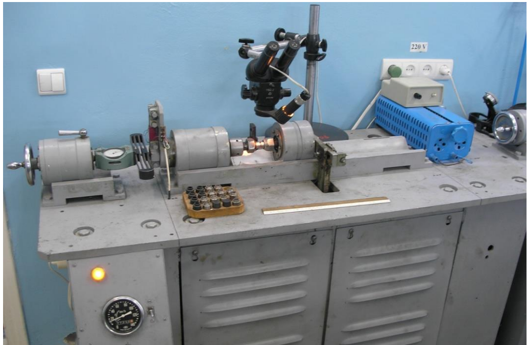
Figure 2.8 – General view of installation MΦK - 1 for testing the fretting
