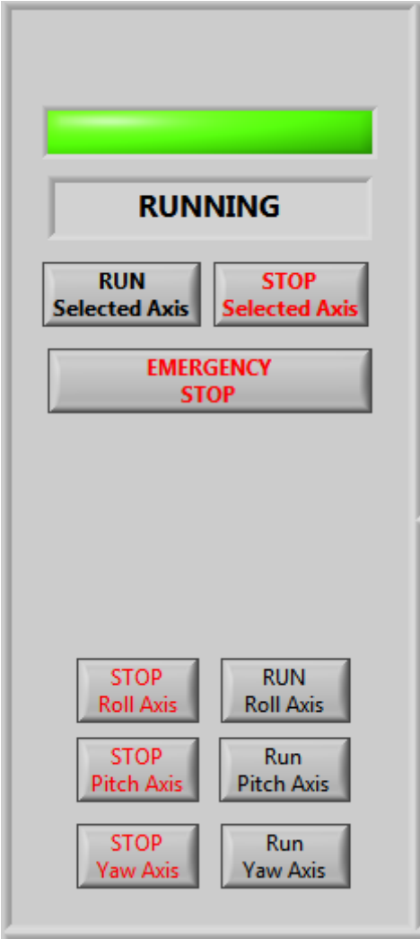
Fig. 3.2 LabView implementation of operation panel
