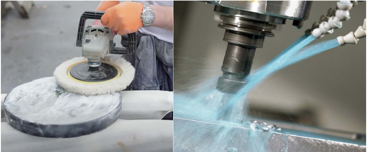
Fig. 4.9. The use of special liquids and pastes in mechanical processing of polymer composites.
