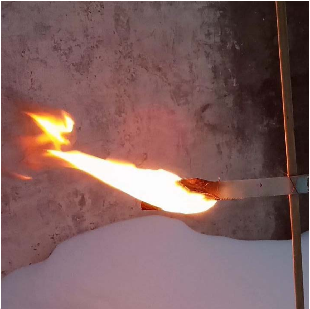
Fig. 4.10. Excellent combustion of polymer composite (fiberglass reinforcing element, matrix resin Larit L-285).
