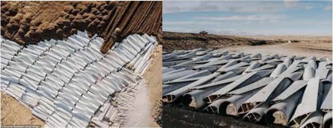
Fig.3.1. Burying wind turbine blades in the ground.
