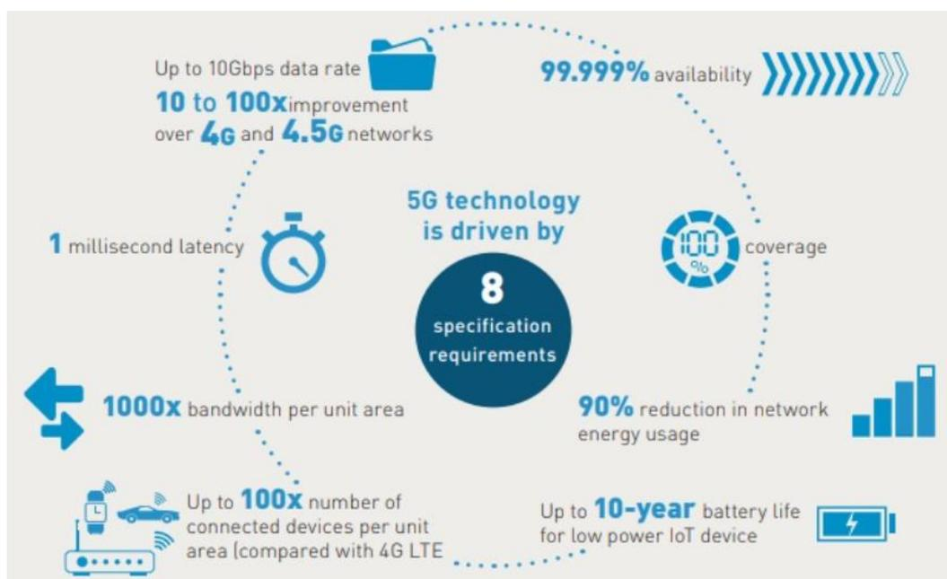
Fig. 2.13. The 8 specification requirements of 5G technology
