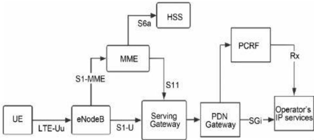
Fig. 2.2. EPS network architecture
