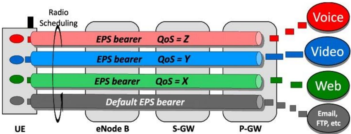
Fig. 2.3. 4G LTE network QoS architecture
