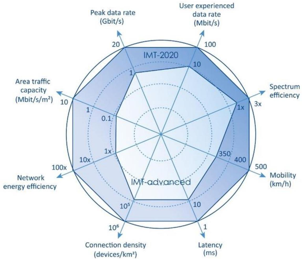
Fig. 2.4. The primary features of IMT-Advanced (4th generation) with IMT-2020 (5th generation) as per ITU-R M.2083
