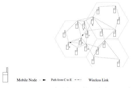
Fig. 1.4. An ad-hoc wireless network
