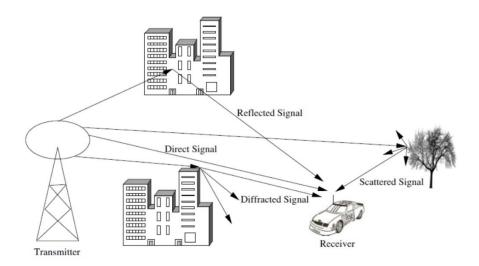
Fig. 1.1. Propagation mechanisms
