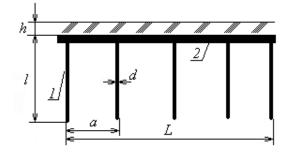
Fig. 5.3. Diagram of the location of grounding devices: 1 – grounding device; 2 – grounding conductor
