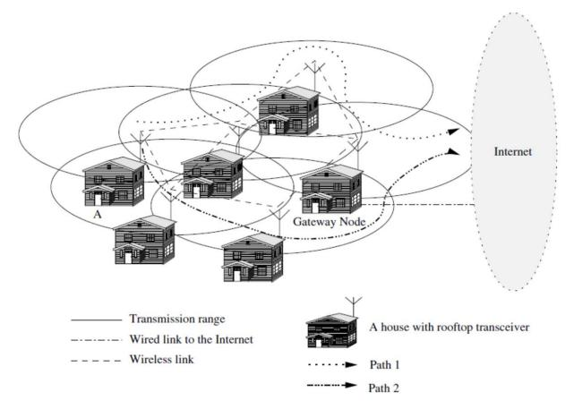
Fig. 1.9. An illustration of the ad-hoc Internet implemented by a wireless mesh network
