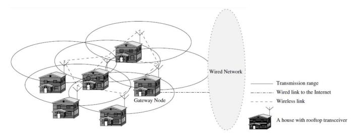
Fig. 1.5. Wireless mesh network operating in a residential zone
