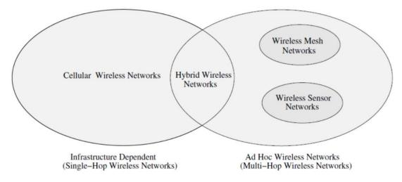
Fig. 1.2. Cellular and ad-hoc wireless networks
