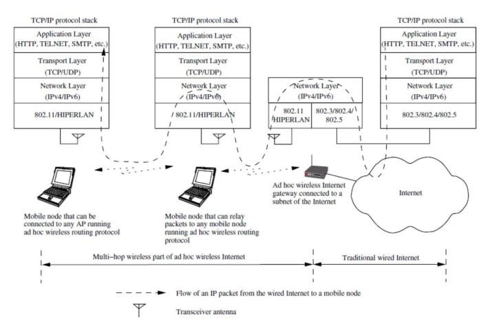
Fig. 1.8. A schematic diagram of the ad-hoc wireless Internet
